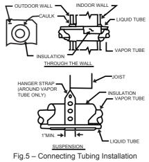
NOTE: Avoid contact between tubing and structure
