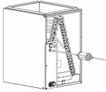
Fig.12—Liquid Line Filter Drier
