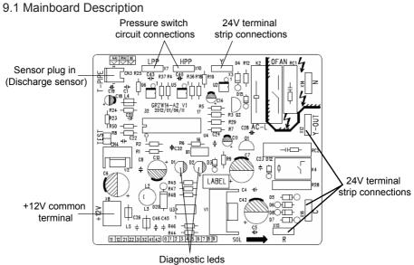
Fig.28 Mainboard Description for cooling only
