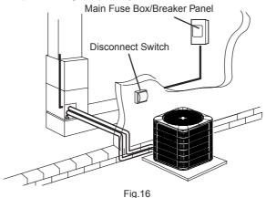
**NOTE:** Units are approved for use only with copper conductors. Ground unit at disconnect switch or to an earth ground.
