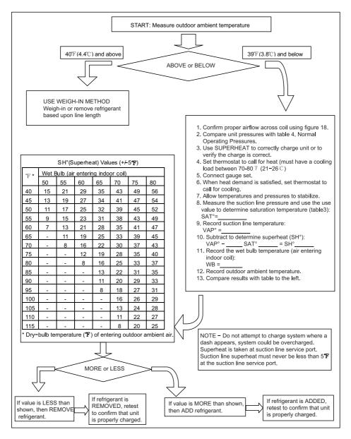
Figure 27. HFC-410A Superheat RFC Method
