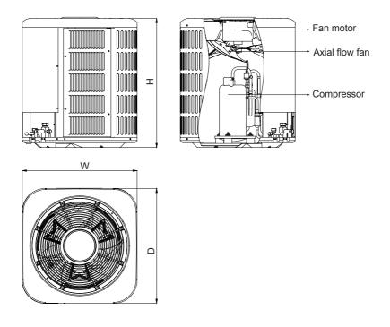
Fig.3—Outdoor Unit Table 1—Dimension of Outdoor Unit
