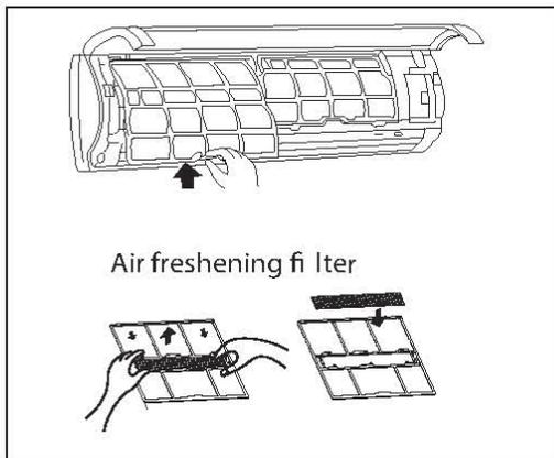
4. Remove the Air Freshening Filter from its supporting frame (on some models).
