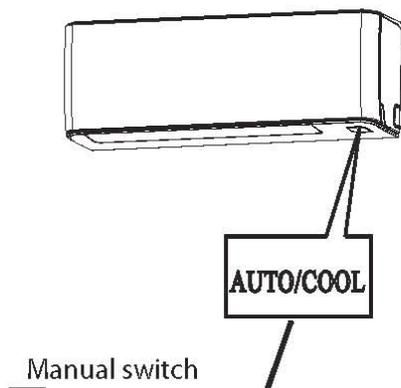
**NOTE:** The unit must be turned off before operating the manual switch. If the unit is operational, continue pressing the manual switch until the unit is off.
