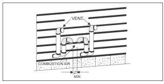
Fig 23: Double Horizontal Combustion Air Intake and Vent Termination
