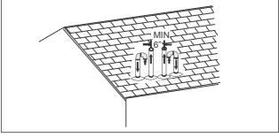
Fig 24: Double Vertical Combustion Air Intake and Vent Termination
