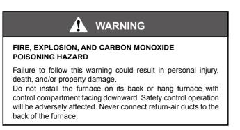
The furnace can be installed horizontally in an attic or crawl space on bottom or either the left-hand (LH) or right-hand (RH) side. The furnace can be hung from floor joists, rafters or trusses or installed on a non-combustible platform, blocks, bricks or pad.
