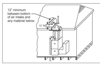
Fig 28: Attic and Crawl Space Combustion Air Termination
