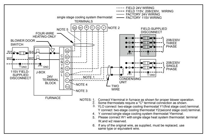
Fig.33 - Heating and Cooling Application Wiring Diagram with 2-Stage heatingThermostat
