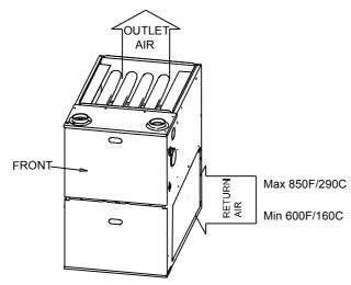
Fig. 3 - Return Air Temperature
