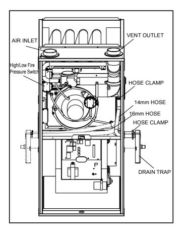
Fig. 11 - Upflow Installation, Top Venting
