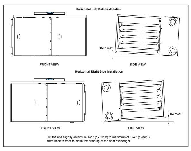
Fig. 7 - Horizontal Application-Setting Equipment
