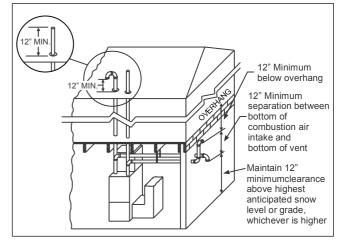
Fig 22: Termination Configuration - 2 Pipe Basement
