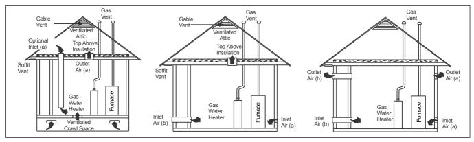
Fig. 27 Outside and Ambient Combustion Air
