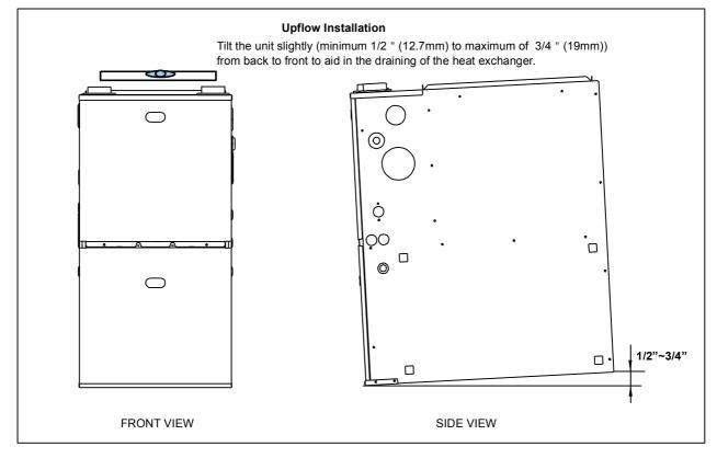
Fig. 6 - Upflow Application-Setting Equipment
