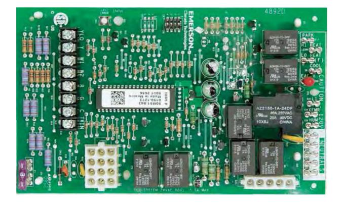
Fig. 32 - Furnace Control
