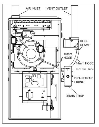
Fig. 12 - Upflow Installation, Right Side Venting
