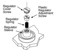
Fig. 34 Gas Valve and Regulator Adjustment
