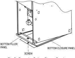
Fig. 5 - Removing Bottom Closure Panel
