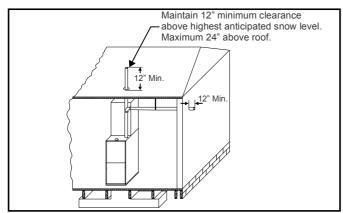
Fig 20: Termination Configuration - 1 Pipe
