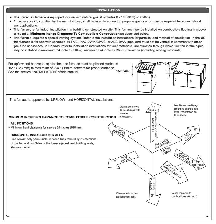
Fig. 2 - Clearances to Combustibles
