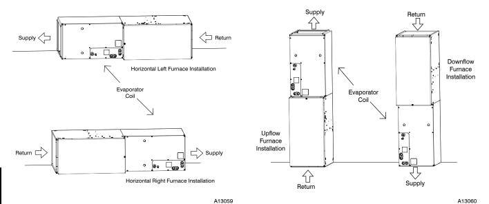
Fig. 1 - Typical Installation Multipoise Cased Coils
