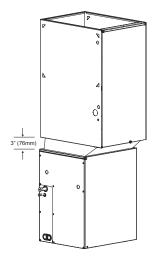
Fig. 3 - Downflow Installation With Coil Rotated 90°
