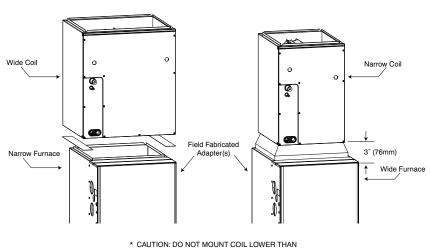
3" (76mm) MINIMUM OR FURNACE FAILURE MAY RESULT
