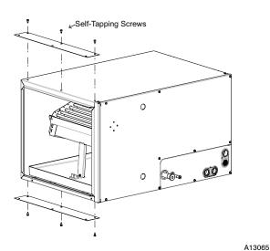
Fig. 4 - Horizontal Right Installation
