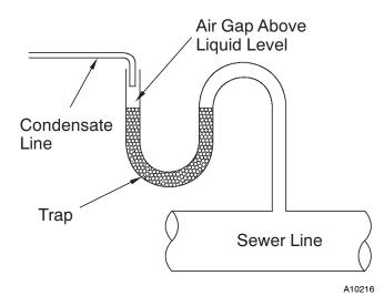
Fig. 9 - Condensate Drain to Waste Line
